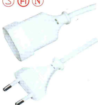
Y001/Y001-Z 欧式延长线 European extension cord 2.5A 250V~ H03VVH2-F 2 × 0.75mm 2 H05VV-F 2 × 0.75mm 2
