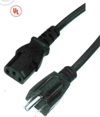
QF3/Q13 电缆组件 American computer connector 10A 250V~ E232289 SJT 18、16AWG × 3C SVT 18AWG × 3C
