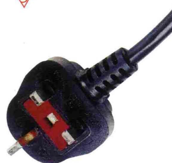
Y006A 英国插头 Britain plug 13A 250V~ BS1363A H05VV-F 3G0.75~1.5mm 2 H03VV-F 2 × 0.5~0.75mm 2 H05VV-F 2 × 0.75~1.5mm 2 H03VVH2-F 2 × 0.75mm 2 H05VVH2-F 2 × 0.75~1.0mm 2 H03RT-F 3G0.75~1.0mm 2
