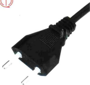
D07 意大利插头 Italy plug 10A 250V~ H05VV-F 2 × 0.75~1.0mm 2 H03VVH2-F 2 × 0.75mm 2 H05VVH2-F 2 × 0.75~1.0mm 2
